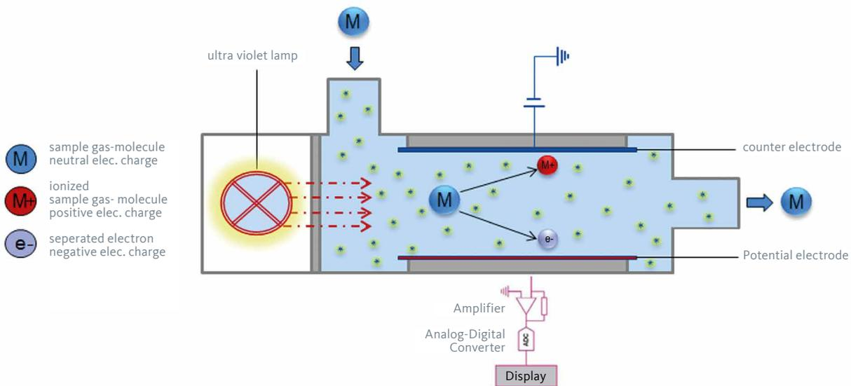
The METPOINT® OCV compact was developed for the detection of steam and gaseous hydrocarbons in compressed air. The detection limit of the measuring method is 0.001 mg/m<sup>3</sup>.
