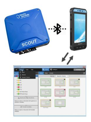
The SCOUT portable connects via Bluetooth to the handheld, which you can then sync with System 1.
