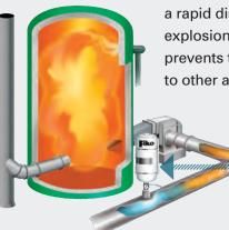
a rapid discharge of a chemical explosion suppressant which prevents the flame from spreading to other areas of the process system.
