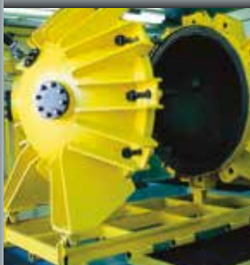
1m 3 laboratory research testing vessel
