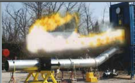
Large scale testing of a Fike mechanical explosion isolation valve
