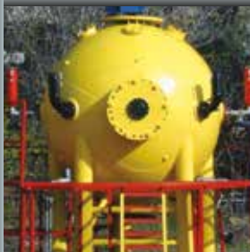
10m 3 sphere for large-scale combustion research
