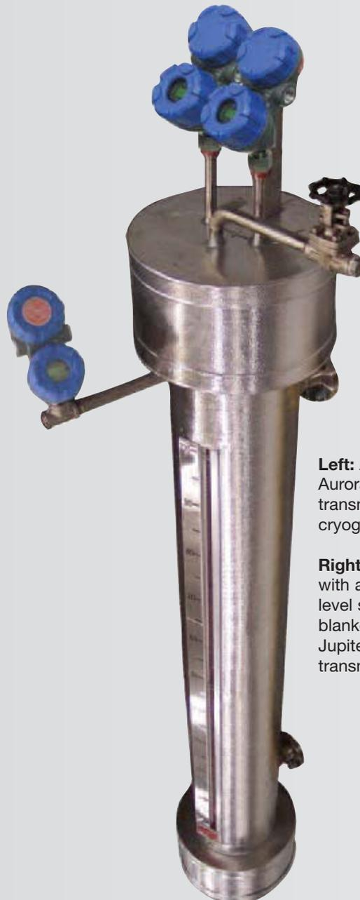
**Left:** A triple-redundant Aurora fitted with three transmitters and special cryogenic insulation.
